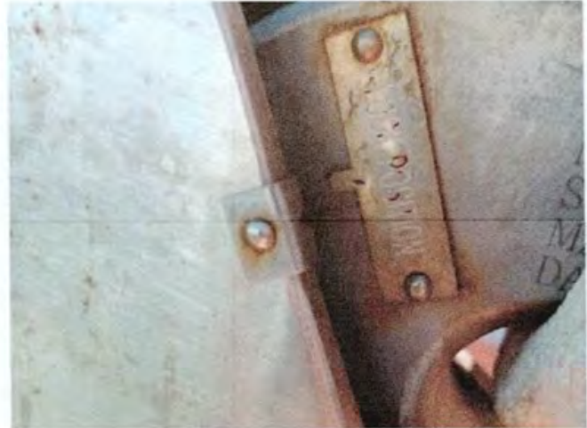
Stbd aft hook indicator not matching before adjustment
