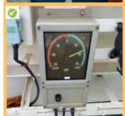
What happened: M/E RPM repeaters on bridge wings were almost unreadable due to the noticeably opaque protective plexiglass.
