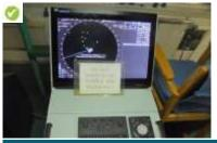
What happened: No warning sign was posted on the ARPA/ RADAR monitor on the bridge while maintenance works were being carried out at ship's mast.
