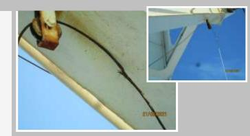
Hazard: Damaged rescue boat wire
