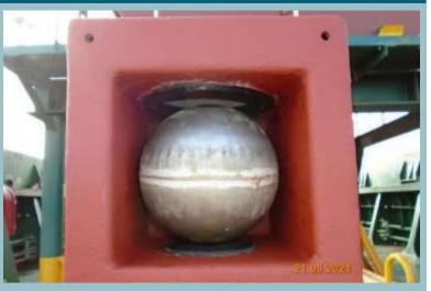
"During the 3months inspection of WBT air vent heads and floaters, the inner coating of vent heads was found in poor condition."
