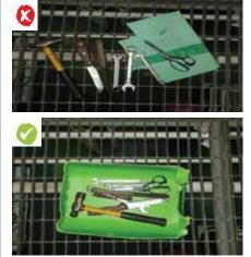
What happened: During repair works, several tools were left lying on the caged floor.
