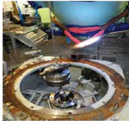
Coupling hub during heating process
