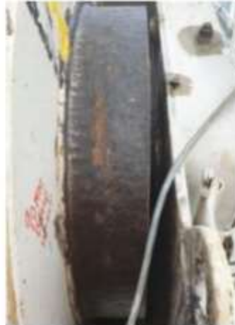
Brake band after descaling
